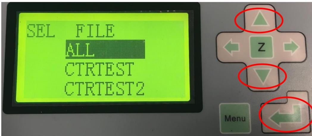
This allows you to select to download **ALL** files from the USB to the machine memory, or to scroll (using the UP / DOWN arrow keys on the machine keypad) to the relevant file name that you want to download, and press the RETURN aka ENTER button to process your selection (the individual file, or all files).
